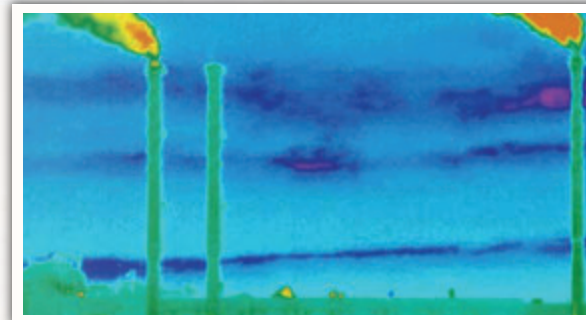
Thermal Cameras detect movement, "see" leaks and temperature variances
